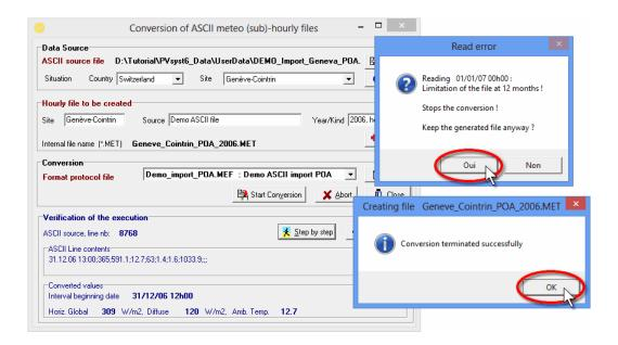
The conversion is now finished and you should carefully check if the result does not contain any obvious error or inconsistency. A prompt asking if you want to open the dialog for visualizing the meteorological data will pop up. Click on "Yes" to open the dialog
