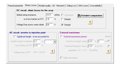
The program proposes a default global wiring loss fraction of 1.5% with respect to the STC running conditions. But you have a specific tool for establishing and optimizing the ohmic losses (press "Detailed Calculation" button). This tool asks for the average length of wires for the string loops, and between the intermediate junction boxes and the inverter, and helps the determination of the wire sections.
