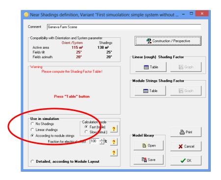
You will be asked once more to compute the shading factor tables, after which you can open the iso-shading graph to compare the results of the improved shadings with the "Linear shadings" case.
