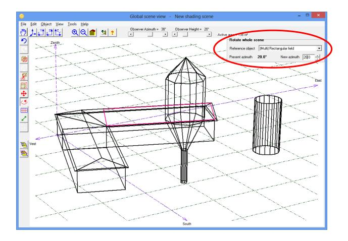
If later on you need to re-position or add a new object in the scene, it might be easiest to rotate back to the original coordinate system. To do this, select an object which is aligned with the coordinate system in which you would like to work and put a value of 0° or 90° into the "Rotate whole scene" dialog. Perform the modifications and then apply the reverse rotation.
