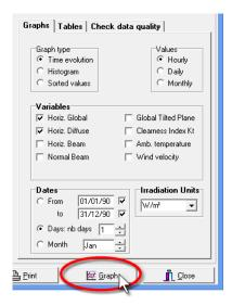
This will open a graph with the hourly meteo values, and you can walk through your entire data using the Scrollbar on the right. The plot includes a blue line, which represents the Clear day model, superimposed on your data. It is very important that the data is not shifted on the time axis with respect to the blue line. This will always be the case for the synthetic data or the data imported from known sources using the "Import meteo data" PVsyst tool.
