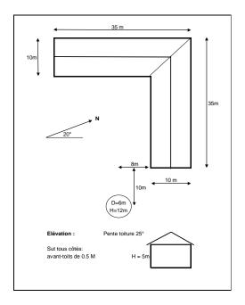
The roof of the farm is facing south and we intend to cover it on an area of about  $5m \times 25 \text{ m} = 125 \text{ m}^2$  with mono-crystalline PV modules.
