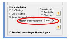
For the simulation that you will present to you end-customer, you can fix a different value to get closer to reality. For the present time there is no means to get a good estimation of this factor (a reasonable guess would be around 60-80%, accounting for a partial recovery due to the by-pass diodes).
