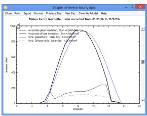
To fix the time shift in the data, two things need to be done: First the data has to be imported again applying the correct time shift. Then PVsyst needs to be told that the data contains a time shift. This is achieved by checking the field "Apply time shift correction" and supplying the corresponding shift value in the field next to it.
