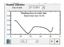
For each time step, the date/hour, sun position and shading factor are displayed on the bottom of the 3D window. You can try this for different dates in the year, the two extreme situations being June 21st and December 21st.
