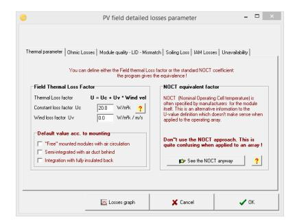
The thermal behavior of the array is computed at each simulation step, by a thermal balance. This establishes the instantaneous operating temperature, to be used by the PV modules modelling.
