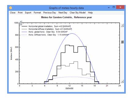
But this may be different for personal data that is imported with the "Import ASCII meteo files" tool. If the data are not matching the Clear day model (i.e. are shifted toward morning or evening), this indicates that the time stamps of the data don't match the PVsyst standard, and all the models using solar geometry will not work properly.
