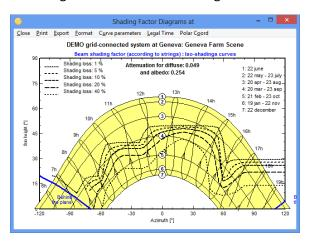
"Fraction for Electrical effect": this is the way how the yellow parts will be treated in the simulation. A 100 % value will withdraw the total electrical production of these areas in the simulation. This is the upper limit of the shading effect. Perform a simulation with this value.
