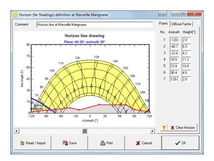
You can either define the horizon line manually. For this the values (Height, Azimuth set of points) have be recorded on-site using a compass and a clinometer (measuring the height angles), a land surveyor or some specific instrument, photographs, etc. But you can also import a horizon line that has been generated with the "SunEye" device or some dedicated software as explained below.
