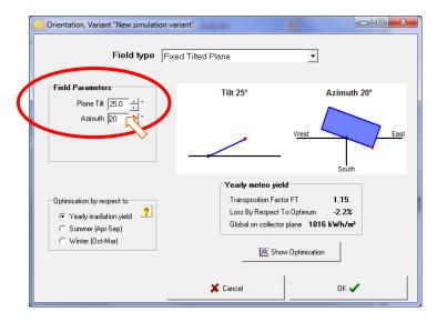
The solar panels in our example will be installed on a fixed tilted plane. From the project's drawing (page 5) we get the Plane Tilt and Azimuth angles (25° and 20° west respectively). The azimuth is defined as the angle between the South direction and the direction where the panels are facing. Angles to the west are counted positive, while angles to the east are counted negative.
