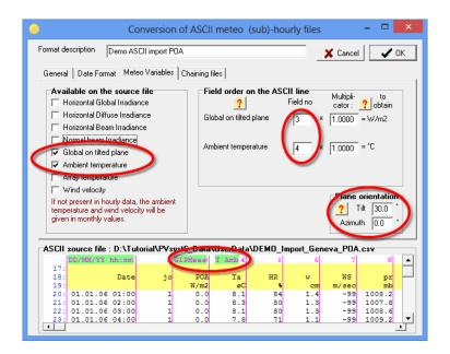
When all the specifications of the format protocol have been entered in the four tabs, click on "OK" and you will be asked to save the newly defined conversion protocol. Give a meaningful description that is not too long to fit in a drop down list. Enter a filename and click on "Save". If a file with the same name already exists you will be asked to confirm to overwrite it.
