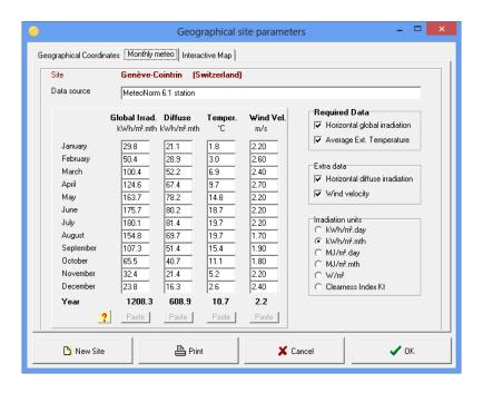
Once monthly data has been imported, the tab "Monthly meteo" will display the monthly values. Values for Global irradiance and Temperature are mandatory input for the simulation. Global diffuse and wind velocity are optional. They will be evaluated by models if and when necessary.
