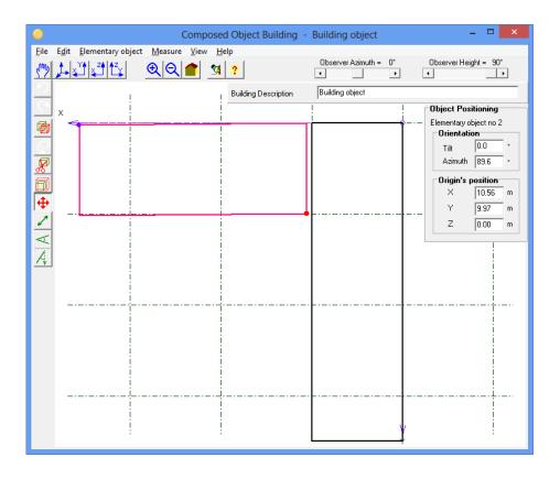
The mouse will not allow you to get precise positioning. But after the object has been placed coarsely, the "Object Positioning" dialog will display the approximate displacement and rotation, and now you can finely adjust the exact values according to the drawing. In our case you will put X = 10.00m, Y = 10.00m, and don't forget Azimuth =  $90.0^{\circ}$
