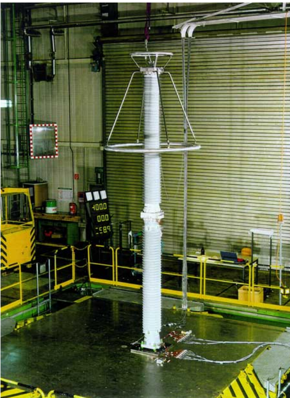
Fig. 21: Polymer housed arrester for a 550-kV-system during seismic testing on a shaking table
